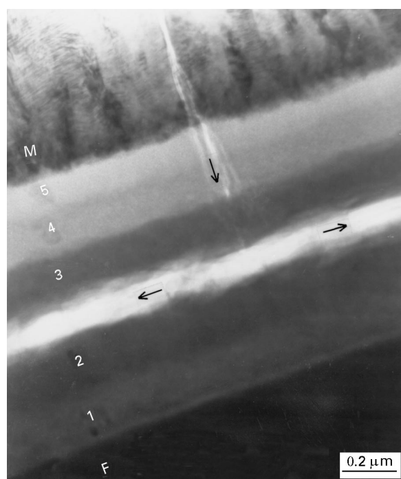
Figure 6 Bright-field image of matrix crack deflection (arrows) in compositional gradient interphase A'. F, fibre; M, matrix; the numbers relate to the five different sublayers involved in the interphase.
